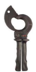
Very solid and easy to use quality cable cutter with a wide range of applications. Blades made out of chrome - nickel steel. Reliable, well proven, needle-roller bearing ratchet drive. All steel parts are hardened. Quick blade release allows fast backout in any position. Can be used even in confined areas.
